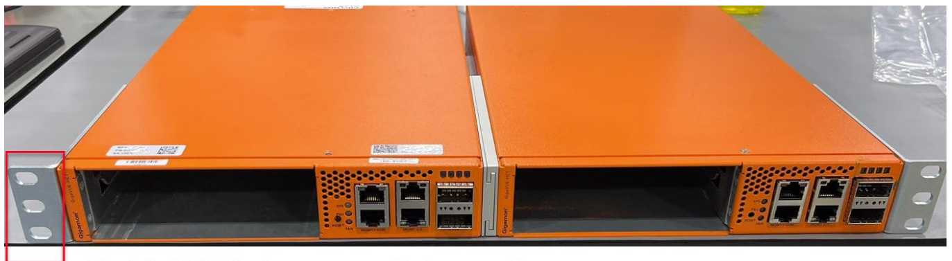
Rack ears face towards the front of the node for Front mounting
