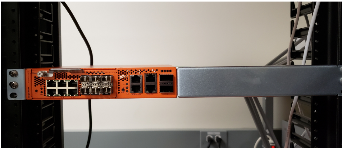
Figure 10 Four-Post Rack Installation (Single Chassis Assembly)
